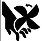
1.f. Do not put your hands near the engine fan. Do not attempt to override the governor or idler by pushing on the throttle control rods while the engine is running.
